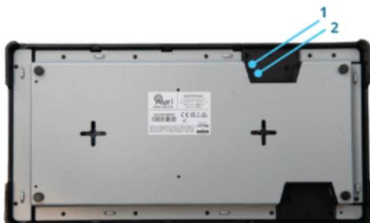
Restart. The device can be restarted through the Auri Manager software, however if it cannot be accessed through the software then it can be reset with a momentary press of this button. Note that this will not change any settings, it is the equivalent of turning the Docking Station off and on again.
